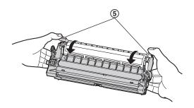
5 Make sure that the triangles (6) match, to install the toner cartridge correctly.
